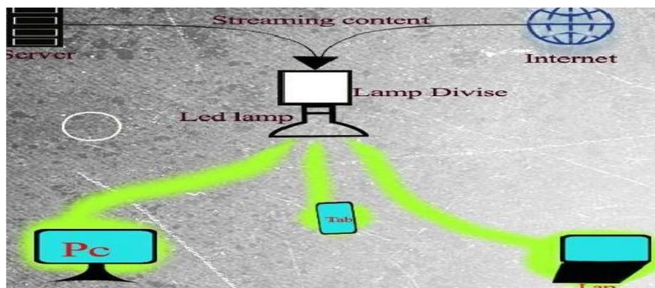
Li-Fi is typically implemented using white LED light bulbs at the downlink transmitter. These devices are normally used for illumination only by applying a constant current. However, by fast and subtle variations of the current, the optical output can be made to vary at extremely high speeds.
